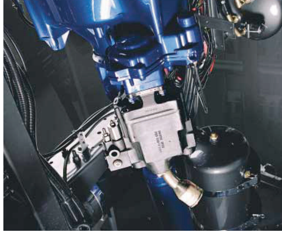
Despite its unique high capacity, the VP1-120 is both light and compact, and can be mounted directly on the PTO without accessories
